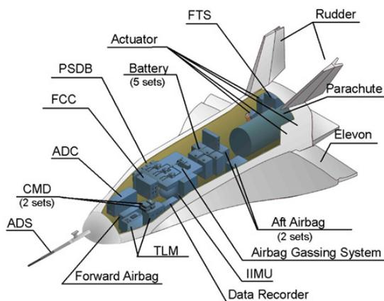
Fig. 13 Phase II vehicle's onboard equipment
