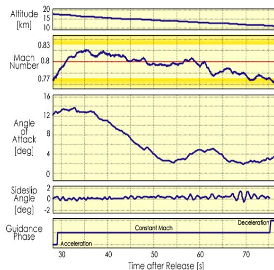
Fig. 16 Flight in the data acquisition phase
