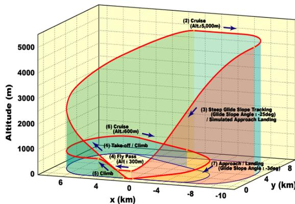
Fig. 10 Flight profile of the third flight
