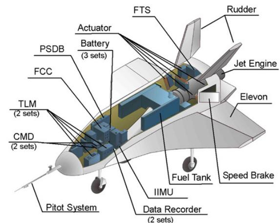
Fig. 8 Phase I vehicle's onboard equipment
