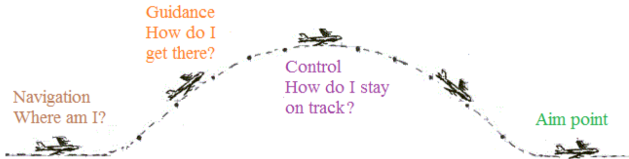
Fig. 1.1 the differences among the concepts of navigation, guidance, and control.
